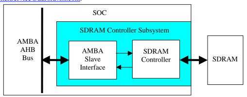
The SDRAM Controller Subsystem supports one, two, or four SDRAM banks (external banks) in SDRAM memory systems through its SDRAM chip select outputs- sdram\_cs[3:0]. The SDRAM data bus, control lines, and clock are common to all banks of SDRAM.
